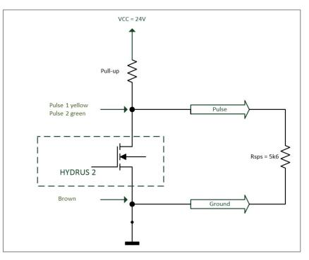
The pulse outputs are wired as open drain.
