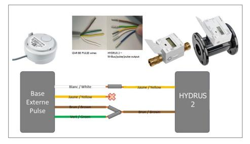
Wiring HYDRUS 2 - Radio/L-Bus/pulse output + IZAR BE PULSE
