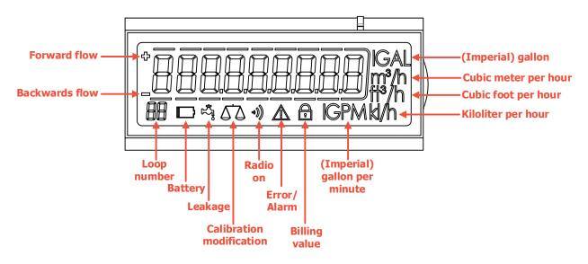
The meter is factory pre-configured with one of the following loops:
