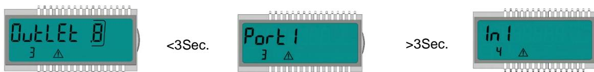
If the button is pressed and held for > 6 s, the meter performs the command shown in the display.
